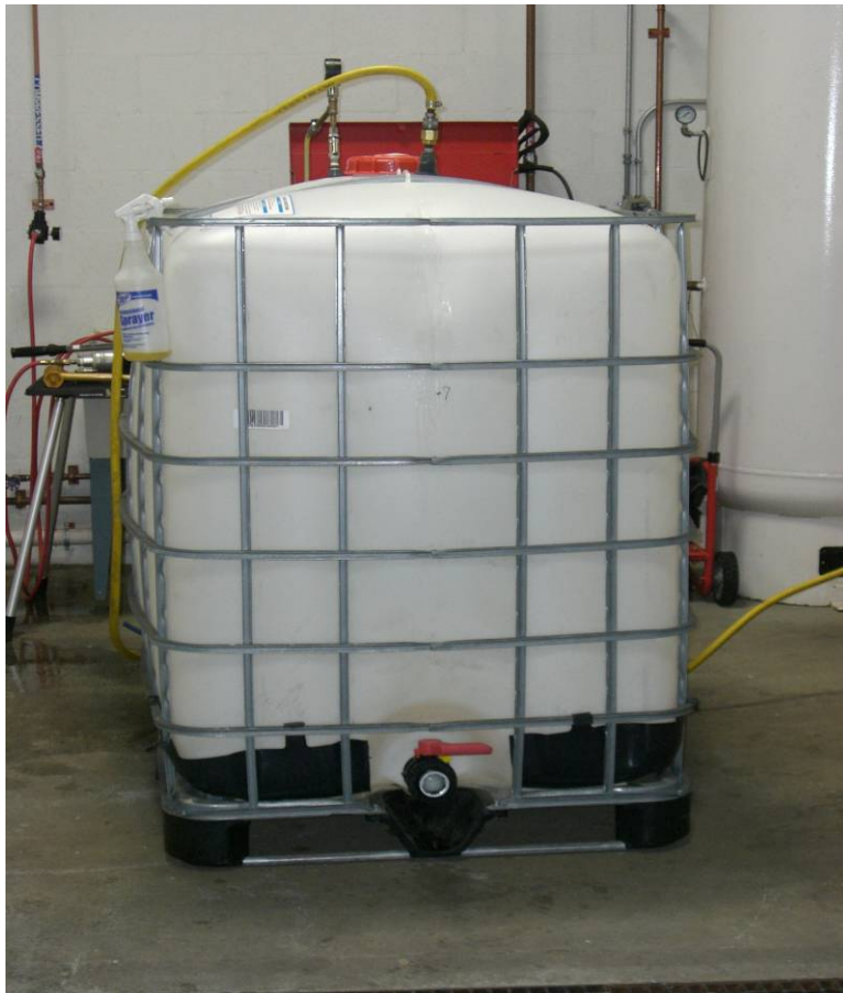
Leakproofness test of 330 Composite IBC. (actual test)
